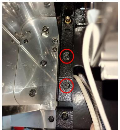
Step 14: Loosen the fixing screw 3mm as the picture shows.
