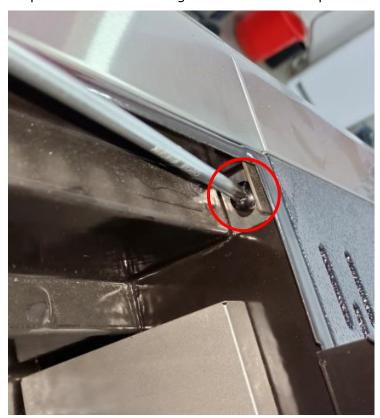
Step 11: Take out the bolts of the side burner injector holder.
