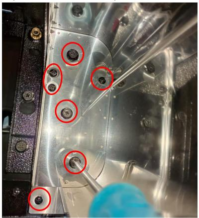
Step 9: Loosen the fixing screws 3mm as the picture shows.
