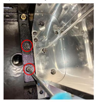
Step 10: Loosen the fixing screw 3mm as the picture shows.
