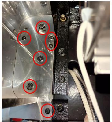
Step 13: Loosen the fixing screws 3mm as the picture shows.
